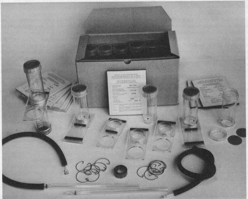
Fig. 2. Test kit for determining susceptibility of adult mosquitoes to insecticides. (Photo furnished by World Health Organization, Geneva, Switzerland).
