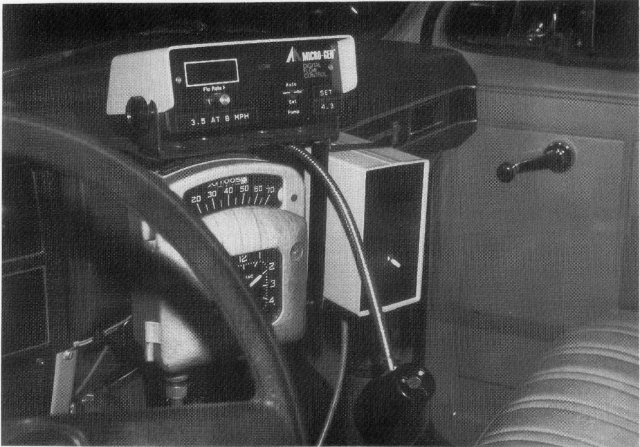
Fig. 3. Location of recorder in vehicle cab adjacent to tachograph and spray equipment control.
