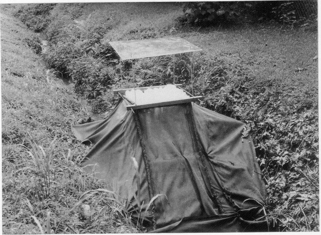
Fig. 1. Photograph of a complete self-marking device positioned over a sewage ditch in East Baton Rouge Parish, LA.
