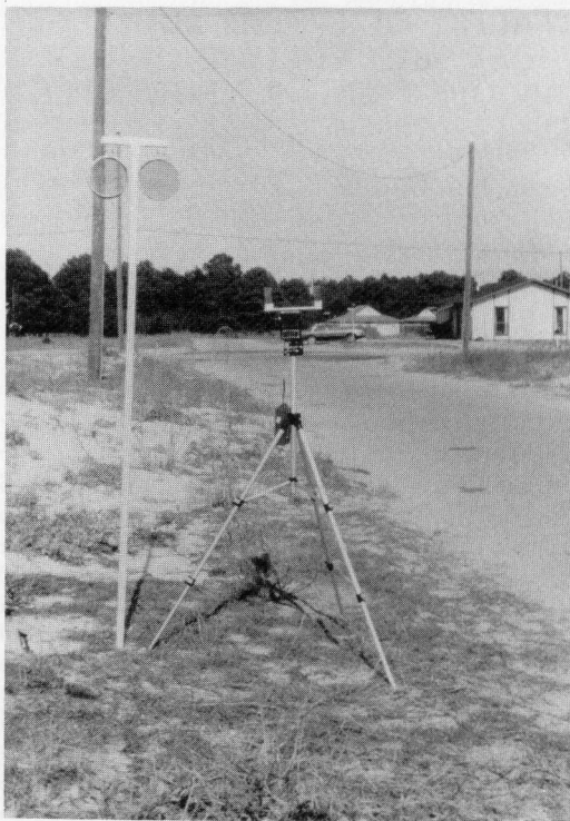
Fig. 1. The open test area with cages of mosquitoes and rotator with slides for sampling droplets.
