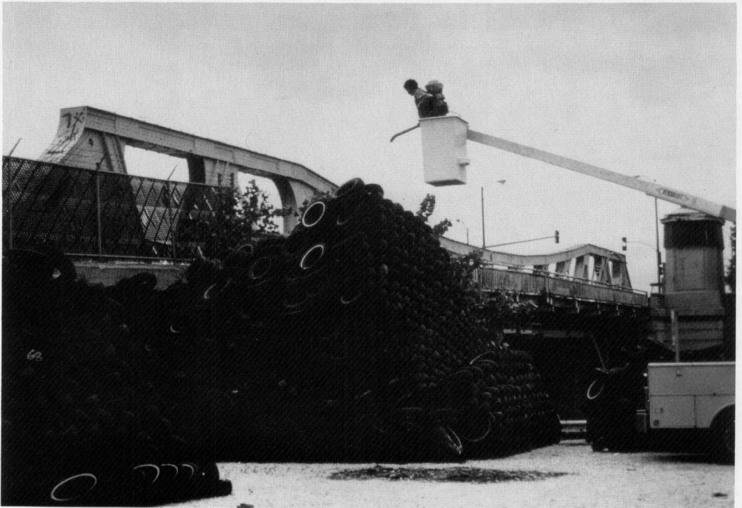
Fig. 2. Application of corncob granules and gypsum pellets using a mobile elevated platform, a "cherry picker."
