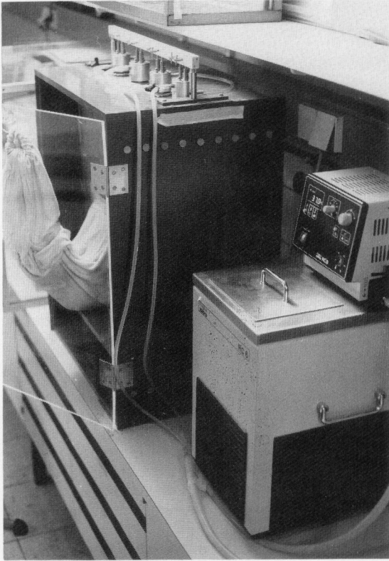
Fig. 2. Feeding system on the rearing cage.
