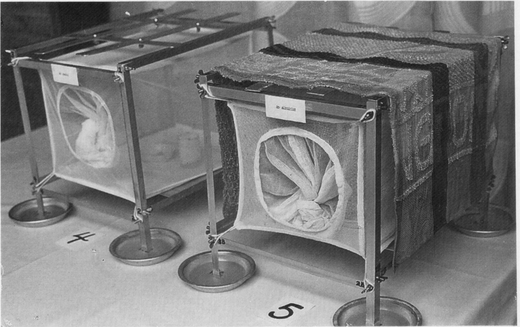
Fig. 3. Completely assembled cage at no. 5 in foreground containing Aedes albopictus . Cage at no. 4 in background with interior exposed to show small saucer and short, wide-mouth bottle inside cage, resting on "floor."
