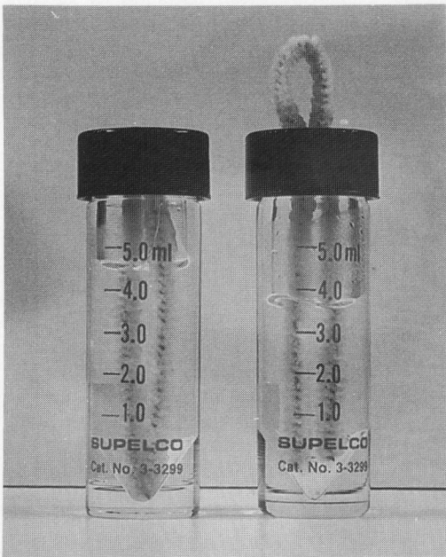
Fig. 1. Octenol is released from vials either through a "wick in" (left vial) arrangement that has a pipe cleaner in contact with a neoprene septum or as a "wick out" arrangement (right vial) that has a pipe cleaner protruding through a neoprene septum.
