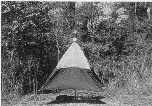
Fig. 1. Tent trap for evaluation of black fly attractants.
