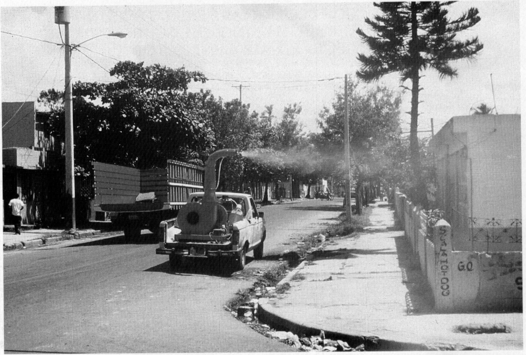
Fig. 1. Use of the truck-mounted, Scorpion™ model 20, ULV forced-air generator in Santo Domingo.
