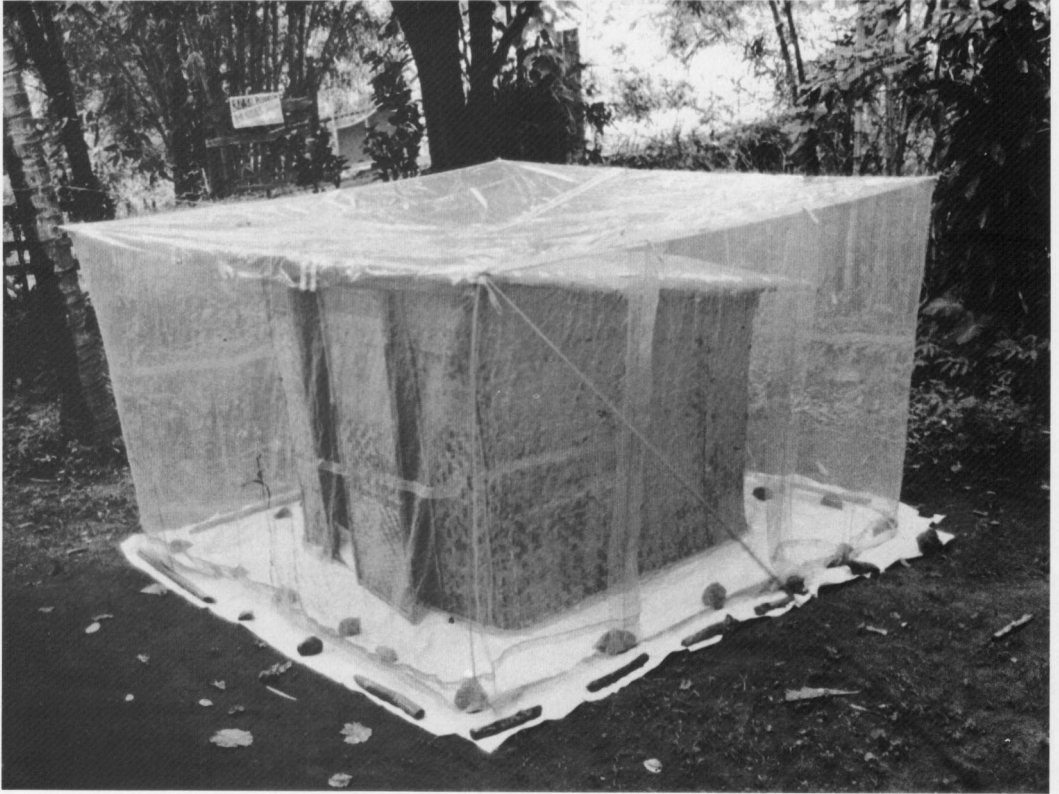
Fig. 1. Experimental hut and mosquito net used to study the mortality of released Anopheles flavirostris exposed to selective or complete spray applications of bendiocarb.
