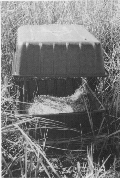
Fig. 1. The oviposition trap with an upper rain shield consisting of a 20 \times 60 \times 90 -cm MacCourt all-purpose tub supported by a 1.27 \times 120 -cm rebar in each corner, and a lower tub of the same type, containing the contaminated towel covered by wheat straw.
