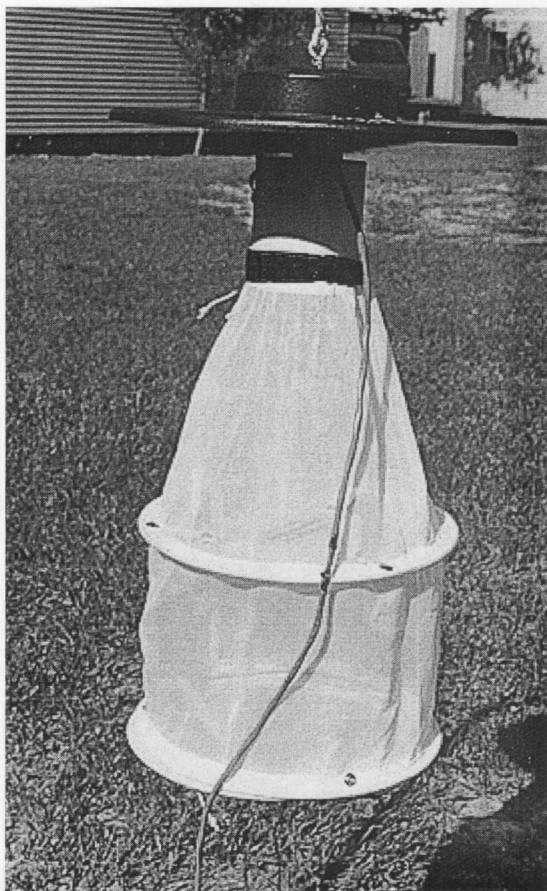
Fig. 1. American Biophysics Corporation (ABC) professional (PRO) trap with CO 2 tank and metering equipment.
