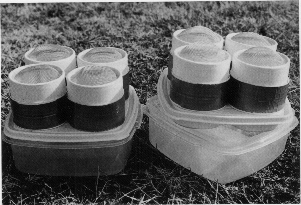
Fig. 1. Two complete MATOCs with aspiration containers installed.
