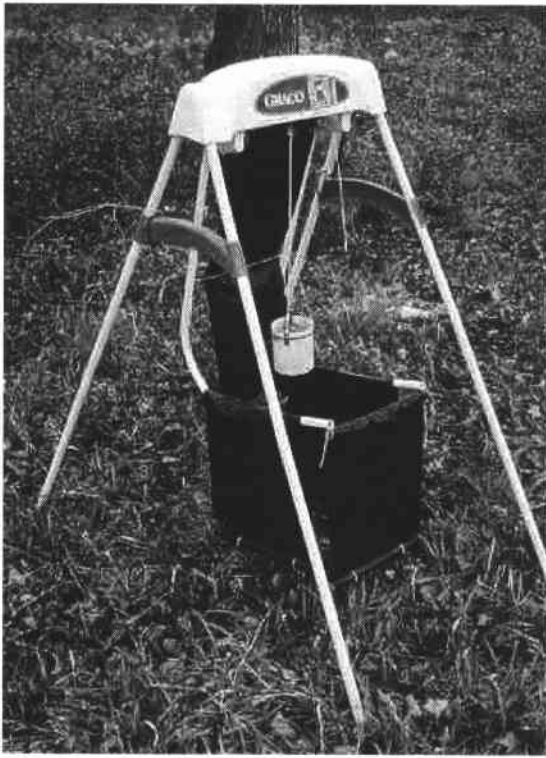
Fig. 1. Moving-target trap fabricated from a battery-powered baby swing.
