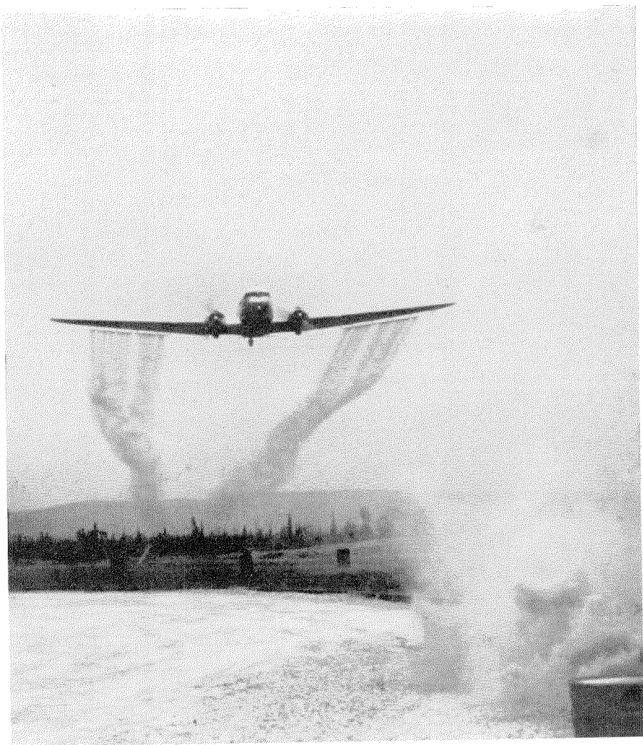
FIG. 2.—C-47 plane distributing spray for the calibration of the equipment.
