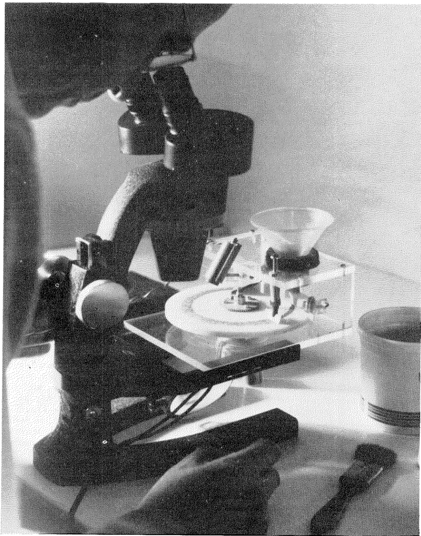
FIGURE 1. Rotary Stage used in the examination of soil samples for the presence of Aedes eggs. Photo T. D. Mulhern
