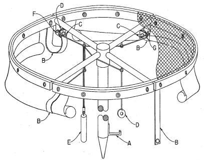
FIGURE 1 : A SCHEMATIC DRAWING OF AN ADULT MOSQUITO SAMPLER.
