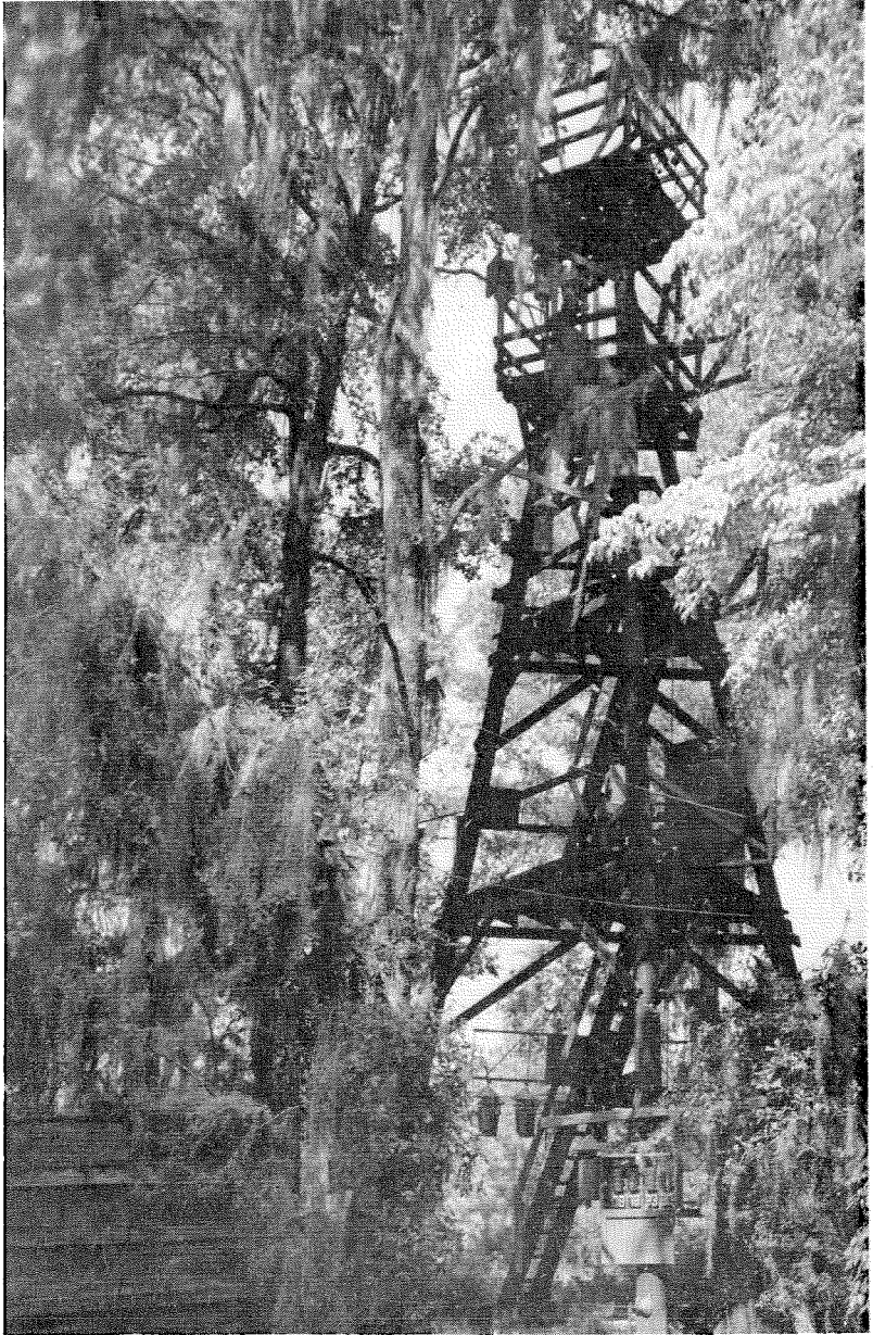
FIG. 1. Tower at Mossy Pond, Baker County, Georgia, used in study of vertical distribution of mosquitoes.
