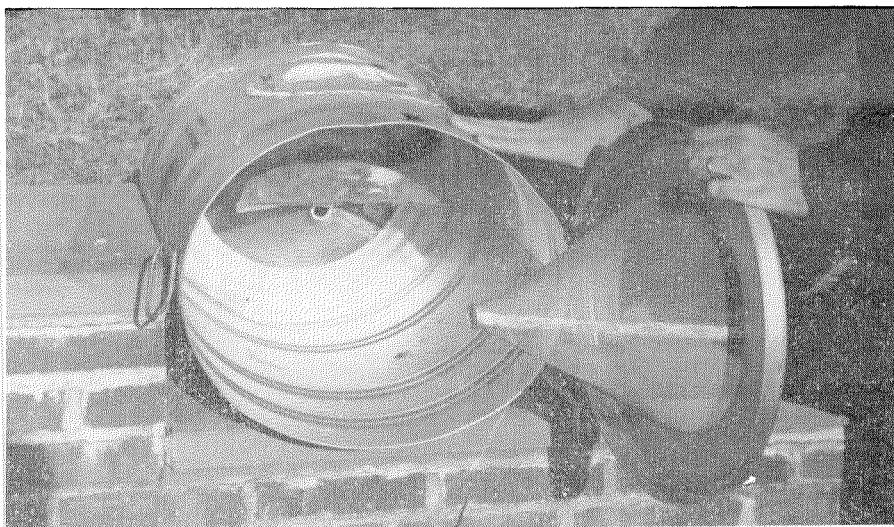
FIG. 1.—Mosquito trap opened at end to show a pigeon in the nylon pocket. The metal cover has been removed from the hole in the top through which the bait is introduced.
