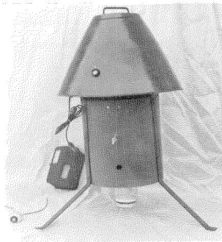
Light trap with electric eye mounted on bonnet of trap. Lower left hand corner is the electric eye and above it the old-fashioned clock.
