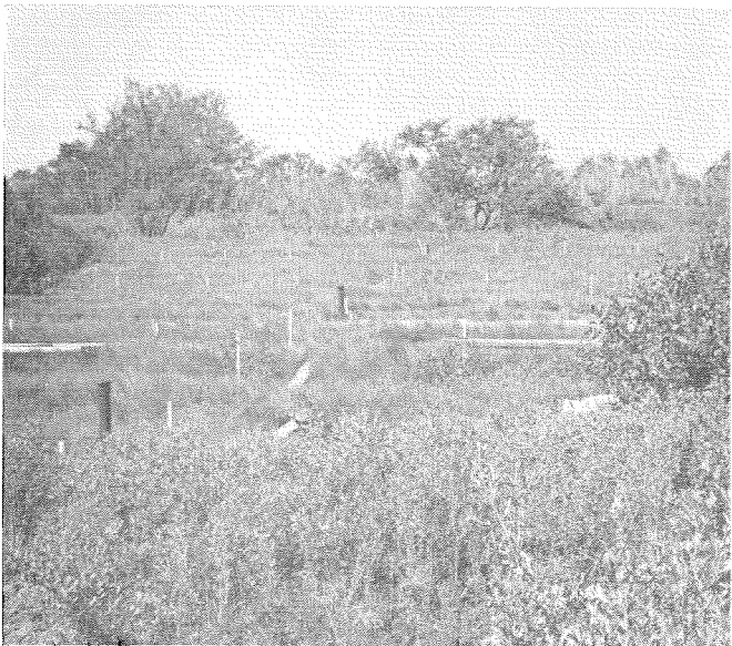
FIG. 2.—Swales showing stakes and well pipes for observation of water levels above and below ground.
