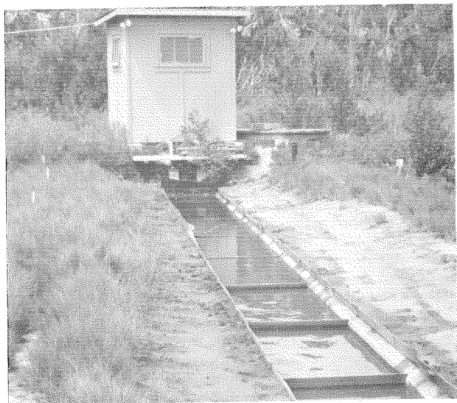
FIG. 3.—The concrete trough with heat-controlled bottom. Separators create 1 x 2 meter cells.
