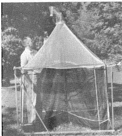
FIG. 1.—Malaise trap in operating position.
