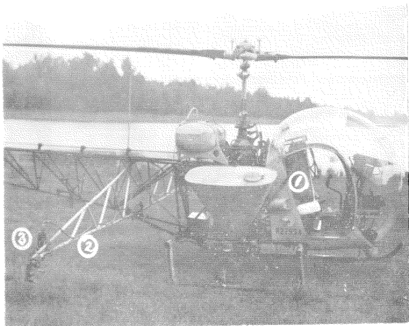
FIG. 2.—Side view of helicopter with experimental spray rig mounted. Legend same as in Fig. 1.
