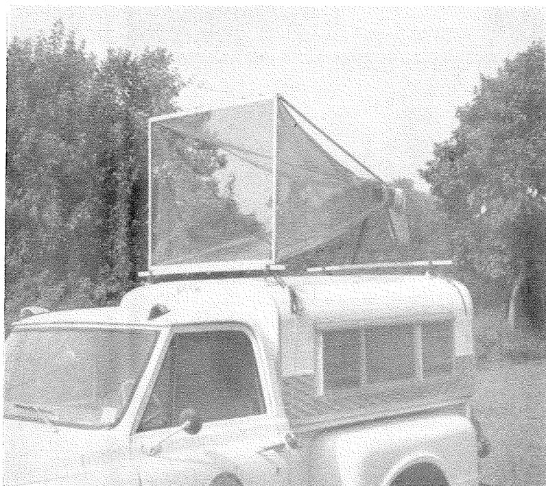
FIG. 1.—Trap mounted on cover of pick-up bed.
