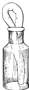
FIG. 3.—Detail drawings of the screen protecting the wick and the dental roll for glucose feeding.
