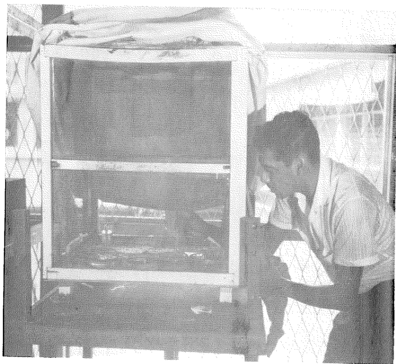
FIG. 3.— Trichoprosopon colony cage. Note oilskin hood lifted back to show interior; also anti-formica cups for cage legs, (Photo Drysdale).
