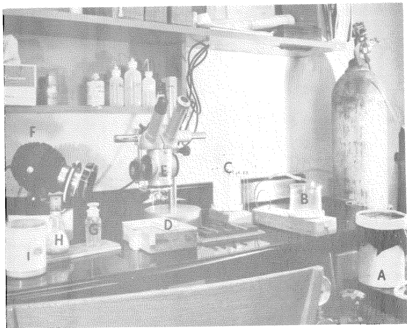
FIG. 1.—Laboratory set-up used for routine induced insemination, showing A, holding cage; B, gas chamber; C, humidity chamber; D, holding block; E, stereomicroscope; F, microscope lamp; G, methyl cellulose bottle; H, etherizer; I, recovery cage.
