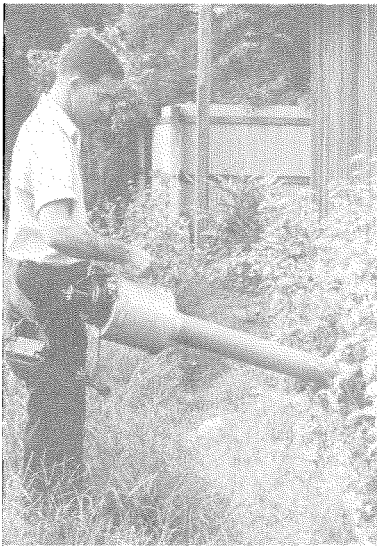
FIG. 3. Suction apparatus being used to collect mosquitoes from vegetation.
