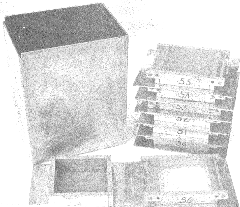
FIG. 1.—A device for the pupal separation of male from female mosquitoes in the field.
