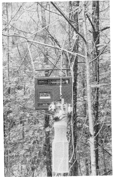
Fig. 1 Modified CDC miniature light trap and cassette recorder in position for collecting female Corethrella .
