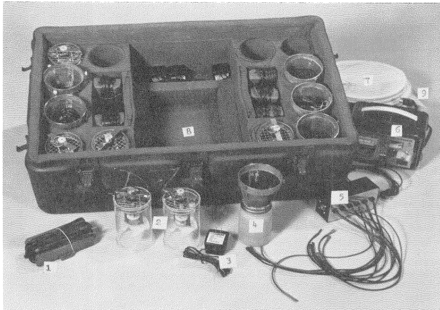
Figure 1. The Army portable insect survey set. (1) D-cell battery holder, (2) AMSS trap, (3) AC/DC converter, (4) Killjar assembly, (5) Charging spider, (6) Battery charger, (7) Catch-nets, (8) Chest, (9) Trap lids under nets. Gel-cell batteries not pictured.
