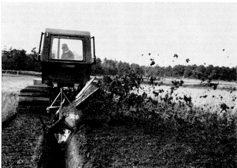
Fig. 2. Dondi Ditcher in operation.
