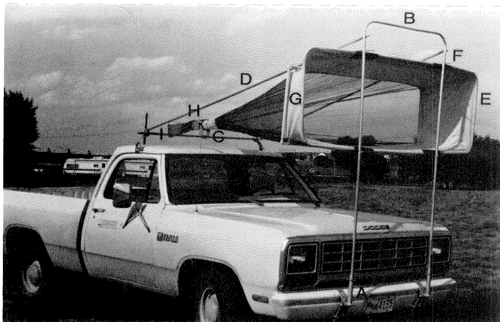
Fig. 3. Vehicle trap mounted and ready for collecting. A. Front bumper supports. B. Front mount. C. Rear mount. D. Lateral brace. E. Internal front bag frame in sleeve. F. Leather reinforcement. G. External front bag frame in sleeve. H. Plexiglas pipe in trap bag cylinder. I. Insect collecting bag.
