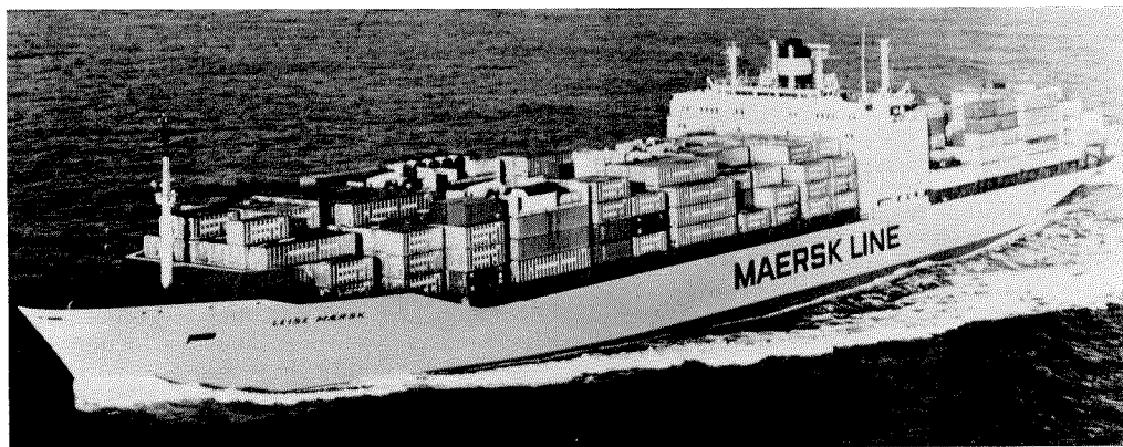
Fig. 2. A typical modern container vessel. Note that many containers are carried above-decks, so that tight seals and good insulation are required to isolate cargo from the elements. Photograph courtesy of Maersk Line.
