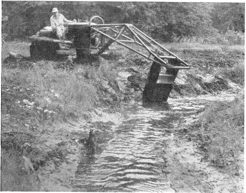
New "Hydraulic Ditching Hoe," now being tested by Mr. James T. Hart, Supt., Morris County Mosquito Extermination Commission, N. J. Designed by Thomas D. Mulhern, N. J. Agr. Expt. Station, \frac{1}{4} cubic yard capacity.
