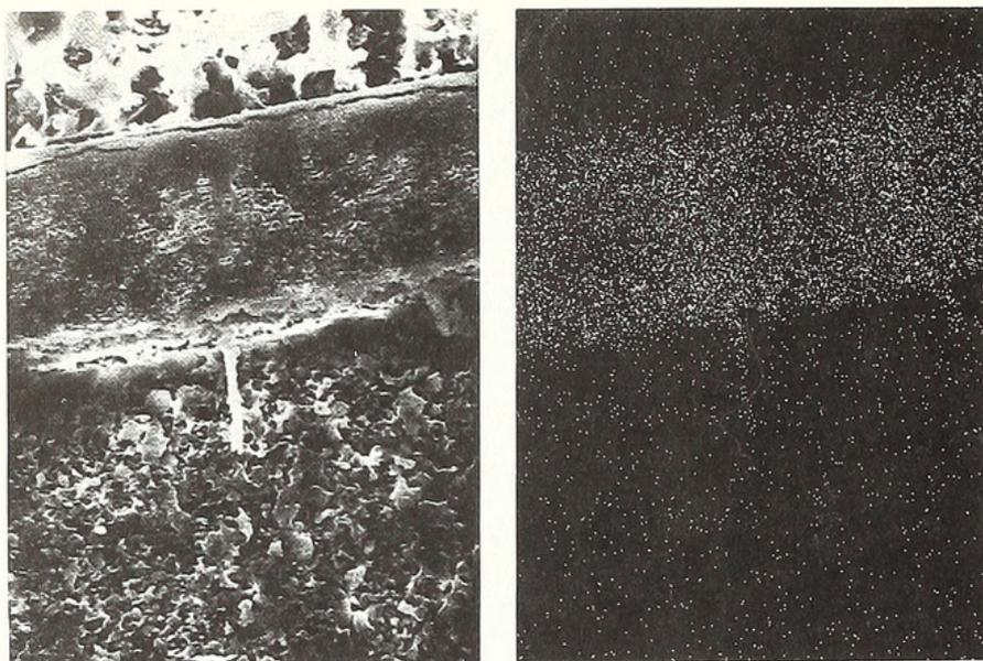
TEXT-FIG. 3. Etched perpendicular section of *Ellipsocephalus polytomus* Linnarsson cuticle outer layer. Left, scanning electron micrograph; right, spot X-ray microanalysis for phosphorus. Preparation RM Ar 46218-A2,  $\times 450$ .
