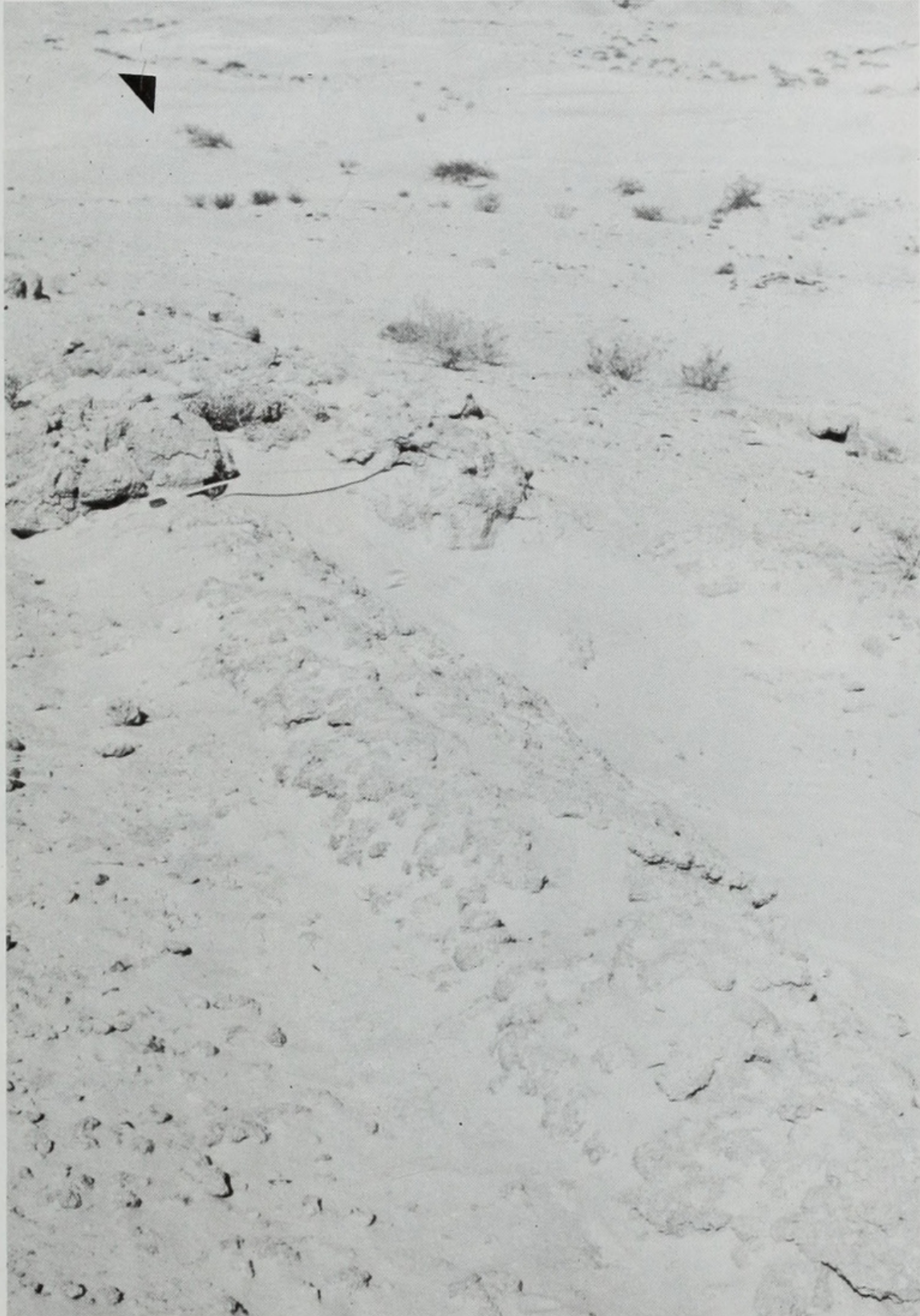
Fig. 6 Similar view to Fig. 4 (photo taken 1979) showing the in situ 'logs'. The drainage channel, shown in Fig. 4, indicates little erosion in over 40 years. Tape = 1 metre.
