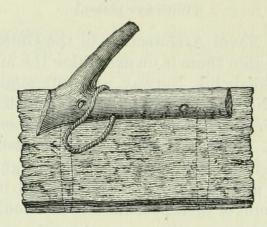
In some fishing craft the planks are tied to the frames by ropes through holes in the under side of the frames and corresponding holes or in cleats projecting from the planks.
