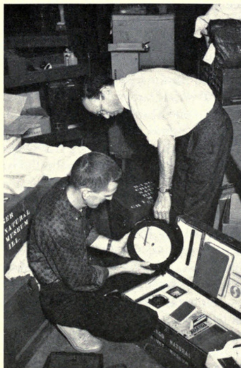
Fig. 3: Thermohumidigraph for recording temperature and relative humidity is placed in field chest for shipment to Borneo.
