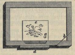
over the object from sliding. Another slip of glass is cemented on the lower side of the cell at d, but not extending as far as the removed part at b. The object of this is to prevent the water in the cell from being removed by capillary attraction, in case the slide in the neighbourhood of b should be a little wetted.
