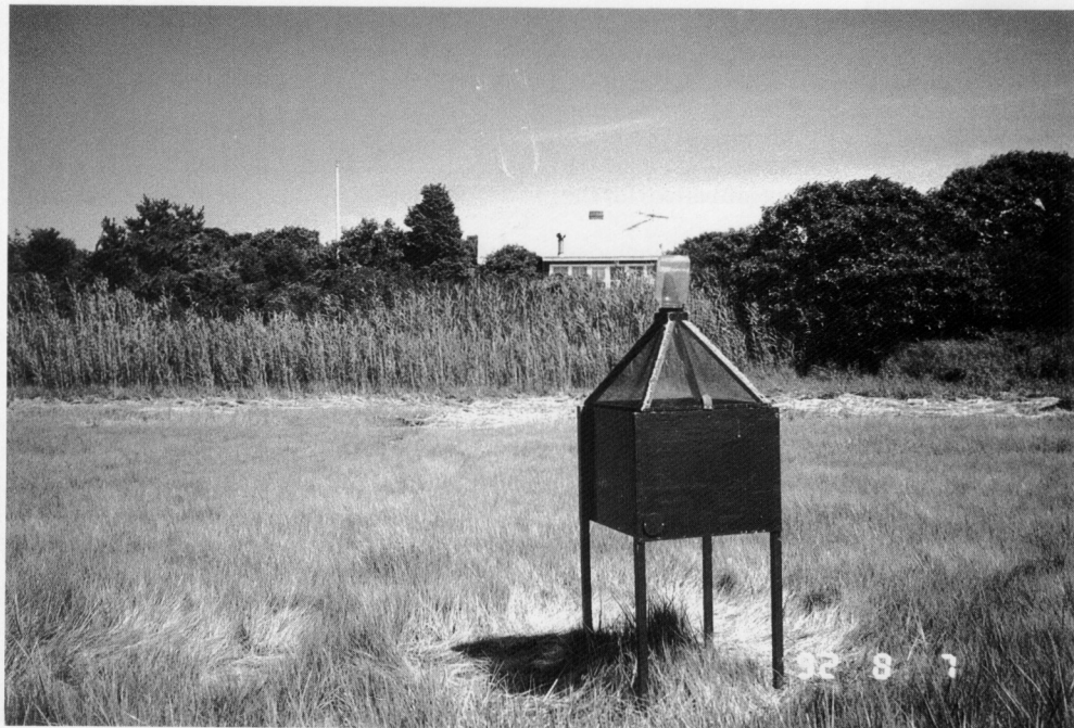
Fig. 1. The pyramid-shaped top attached to a box trap on the salt marsh was useful for collecting, concentrating, and removing trapped tabanid flies.
