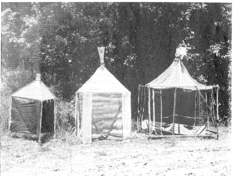
FIG. 2.—Triangular trap (left), Kerrville Malaise trap with natural saran screen (center), and TVA Malaise trap (right).
