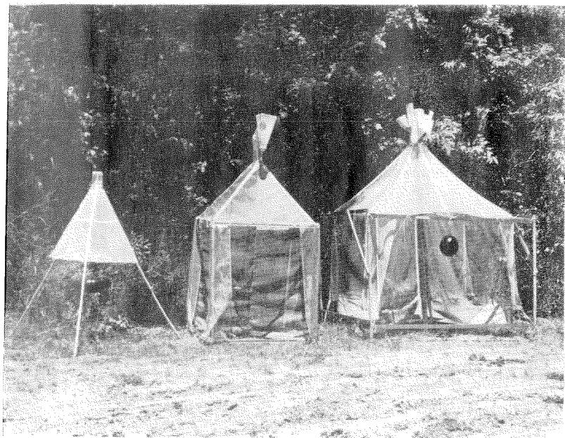
FIG. 3.—Manitoba fly trap (left), Kerrville Malaise trap with gray screen (center), and Stoneville Malaise trap (right).
