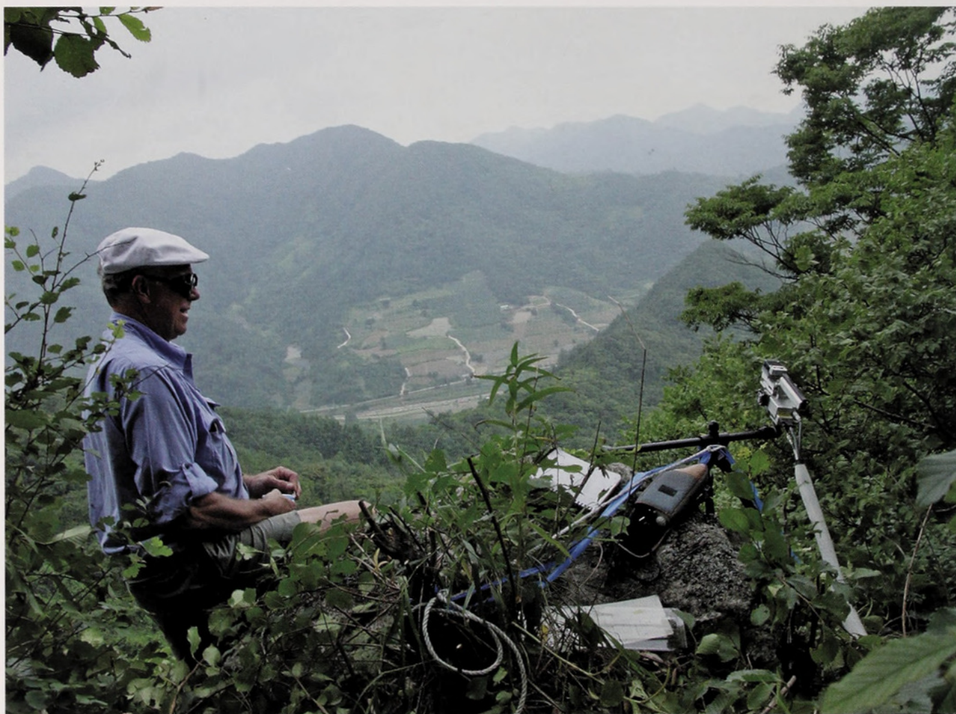
Tom Whitlow uses the LiCor 6400 to measure photosynthesis on a tree growing near the Buddhist hermitage at Podogam on Woraksan. The real-time photosynthetic rate (expressed as the rate of \text{CO}_2 ) is determined after inserting a leaf in the unit's cuvette, seen attached to a tripod on the righthand side of the image.
