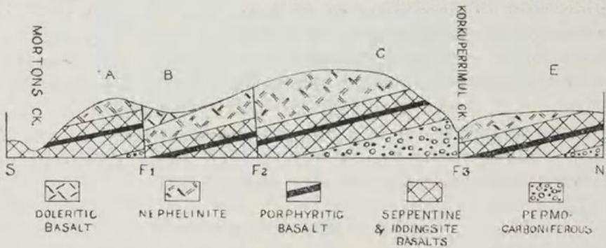
Fig. 7.—A diagrammatic north-south section showing the Older Basalt lava sequence along the Korkuperrimul Creek. The faults  $F_1$ ,  $F_2$  and  $F_3$  are described on pages 112-113. The length of the section is approximately  $1\frac{1}{2}$  miles.
