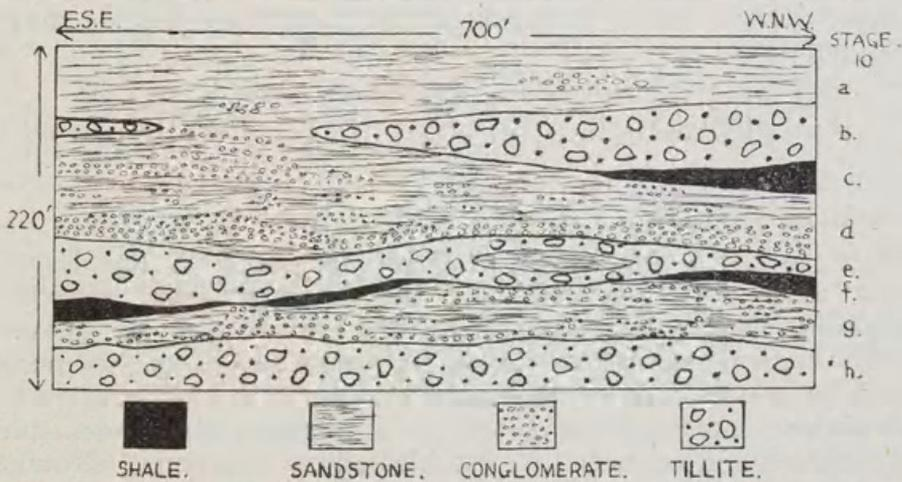
Fig. 5.—Reconstructed vertical section along the strike of the beds of Stage 10, North Korkuperrimul area, showing the extent of lateral and vertical variation.
