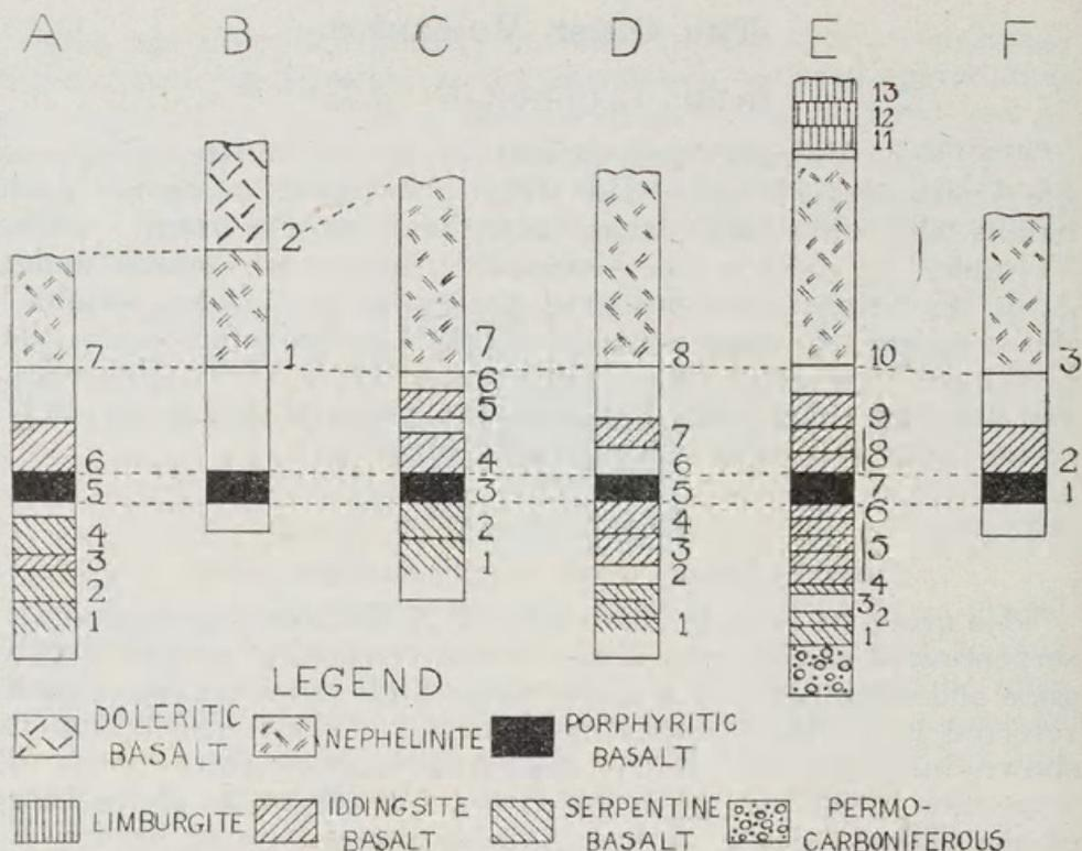
Fig 6.—Shows the detailed lava sequence at six localities, Sections A to F, shown on the map. Approximate vertical scale, 0.66 inches equals 100 feet.
