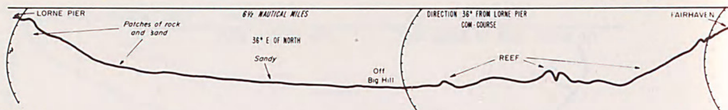
Fig. 3.—Sonar trace B1 parallel to the shore from Lorne to Fairhaven.
