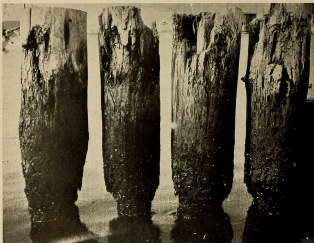
FIG. 41. DESTRUCTION BY MARINE BORERS
