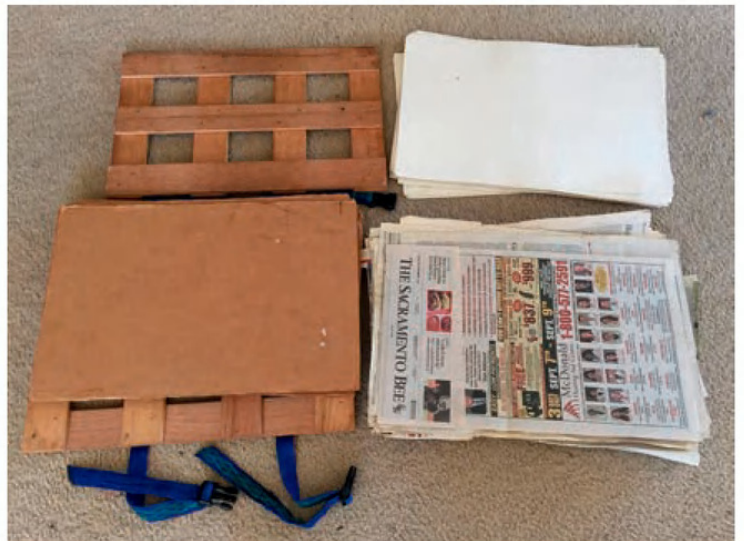
Figure 1: An exploded view of an herbarium press. At left, the wooden frame, straps, and cardboard dividers; bottom right, newspapers; top right, blotter paper.
