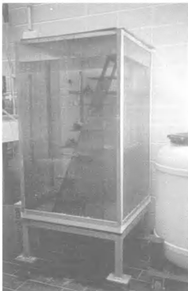
FIG. 1. A 200dm 3 air-lift bioreactor for maintaining the culture of P. andrewsi .
